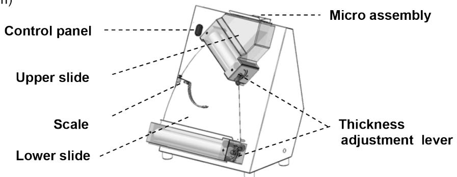
The machine is ideal for rolling pizza dough for pan baking.
