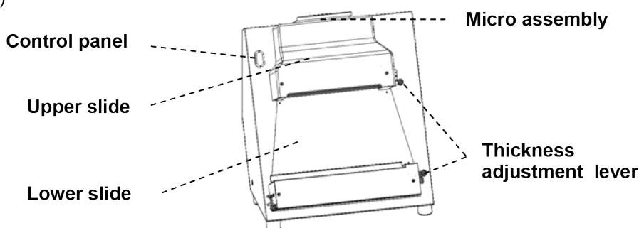
The machine is ideal for rolling pizza dough for pan baking.
